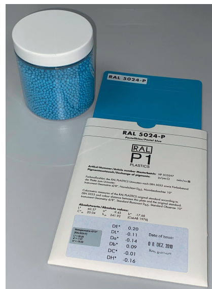
Fig. 2. RAL color charts serve as references for the analyses. © Sensor Instruments
